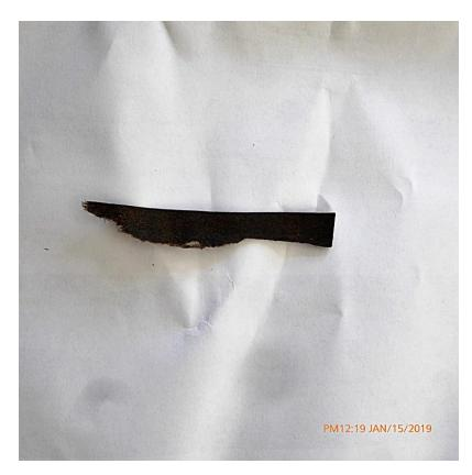
This piece of joint flashing felt was found hanging behind a loose plank.
